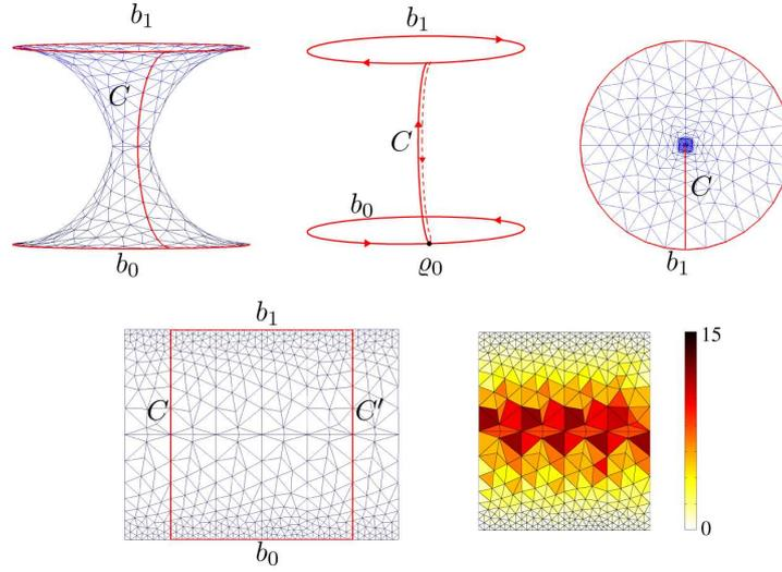
Fig. 2. Example of conformal flattening. Top left: three-dimensional triangular mesh approximating a non-planar test domain. Top center: the oriented boundary  $B$ . Top right: the annulus generated by the flattening procedure. Bottom left: the planar triangulated domain obtained as a final product of the conformal flattening of the test domain. Bottom right: colormap of the quantity  $\mathcal{D}(u)$  associated with the conformal flattening map.
