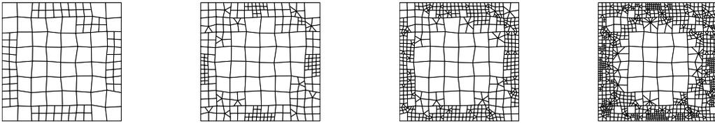
**Fig. 2** First four levels of computational meshes generated by the adaptive refinement strategy employing the fixed fraction marking strategy.
